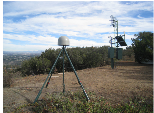
Figure 2. Monument and antenna (under the dome) of a typical cGPS station for monitoring tectonic plate boundary deformation (section 4) and atmospheric water vapor (section 6.1.3), in La Jolla, California. The small white box on the vertical leg contains a MEMS accelerometer used for seismogeodesy (section 5.2.3). See also figure 7 for a schematic of the monument. In the background are GPS equipment enclosures, solar panels, radio antenna for real-time transmission of data, and meteorological instruments. Photo courtesy of D Glen Offield.
