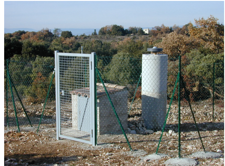
Permanent GPS site, antenna on concrete pillar anchored in bedrock
