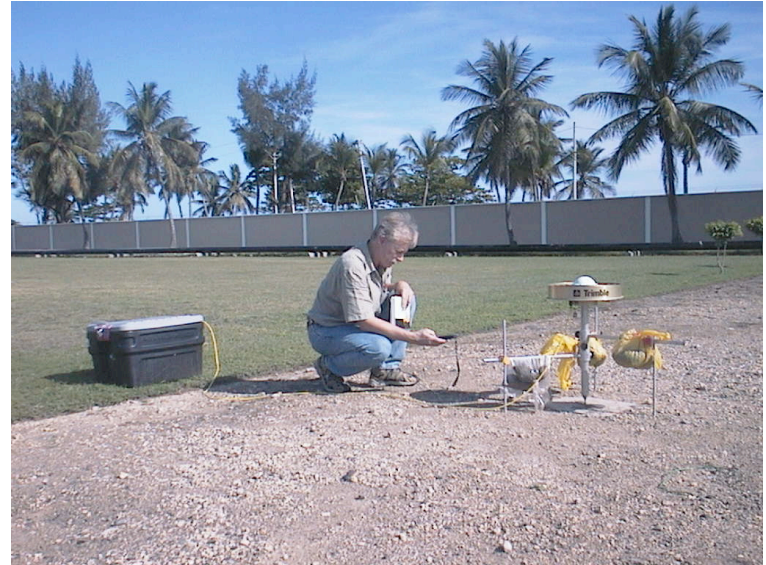
Typical GPS campaign setup using a “spike mount”, Dominican Republic
