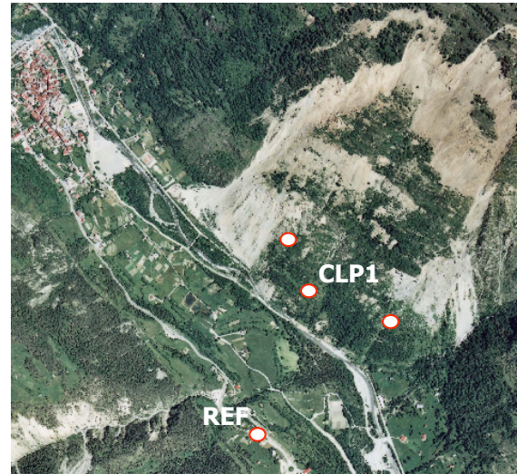
The La Clapiere landslide in the French Alps ( 50 \times 10^6 \text{ m}^3 ). Circles show location of GPS sites
