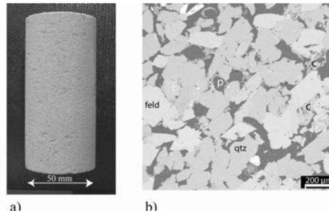
**Figure 1.** a) Picture of a non-deformed sample of Bleurswiler sandstone. b) SEM micrograph (backscattered) of intact sandstone. Epoxy-filled pores (p) appear in black, porosity is about 25%. Quartz, feldspar, and clay are denoted by qtz, feld, and c, respectively.
