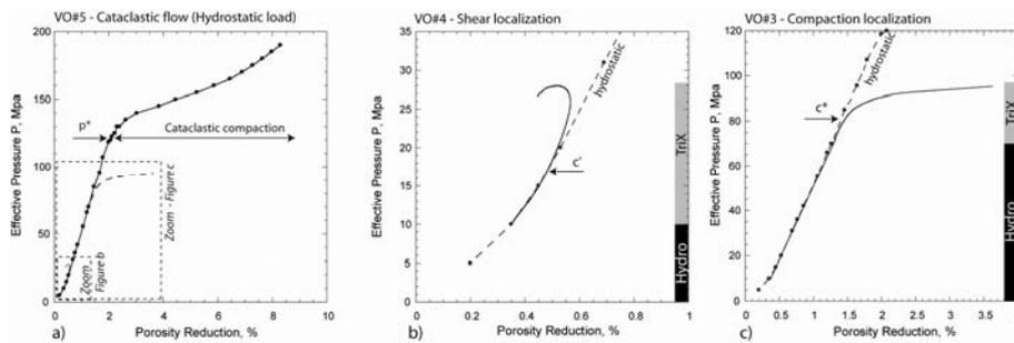
**Figure 3.** Effective mean pressure versus porosity reduction. a) Hydrostatic loading (for reference, the two triaxial experiments are shown as the dashed lines). b) and c) Triaxial compression experiments performed at effective confining pressure of 10 MPa and 70MPa, respectively (for reference, the hydrostatic loading is shown as the dashed line). The critical stress state  $P^*$ ,  $C'$  and  $C^*$  are indicated by arrows.
