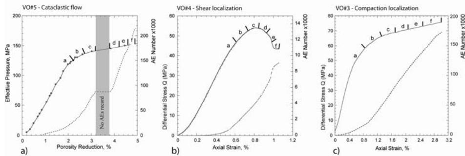
**Figure 4.** a) Hydrostatic experiment: Effective pressure (solid curve) and cumulative AE (dotted line) as functions of porosity reduction. b) and c) Triaxial experiments : differential stress (solid curve) and accumulative AE (dotted line) versus axial. Effective confining pressure was 10 MPa in Figure b) and 70 MPa in Figure c). Six intervals are defined for each experiment (a to f) corresponding to the AE hypocenter distributions shown in Figure 5.
