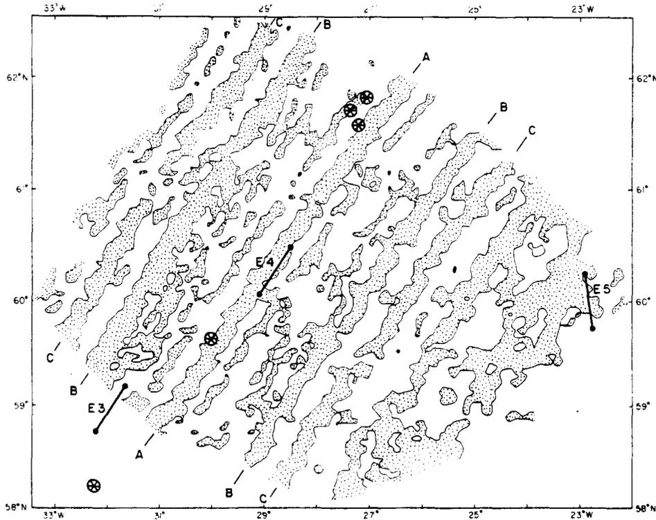
Fig. 7. The magnetic pattern over the area surveyed. Areas of positive anomalies from Fig. 5a and b are shaded. Short line segments are locations of seismic refraction sections shown in Fig. 8. Circles represent earthquake epicenters.
