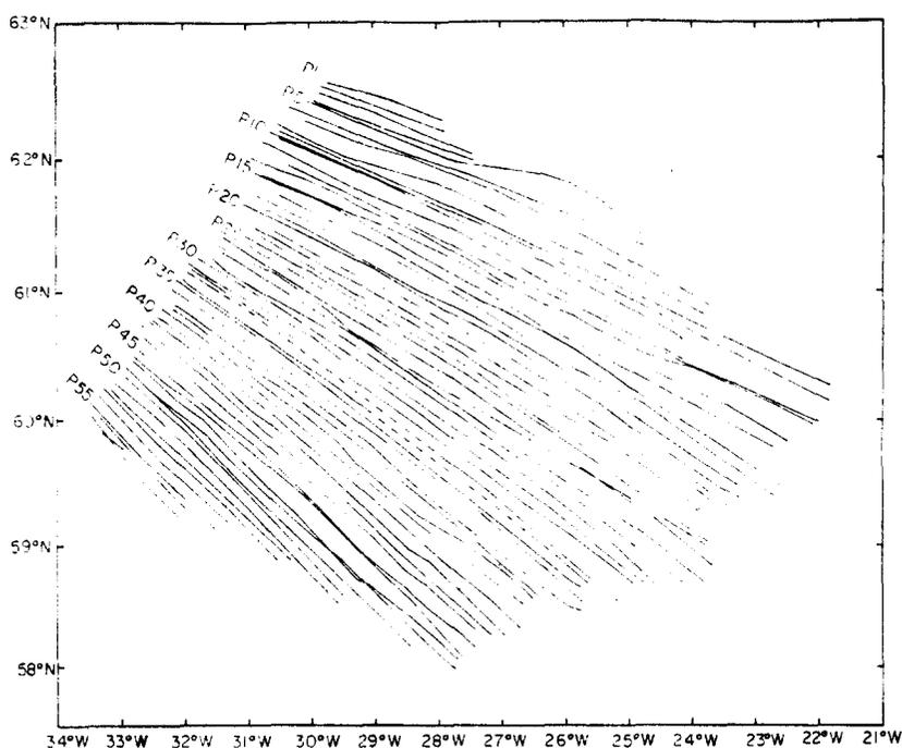
Fig. 2. NW-SE flight lines. Magnetic profiles shown in other figures are identified by the letter "P." Dashed line indicate no magnetic data.
