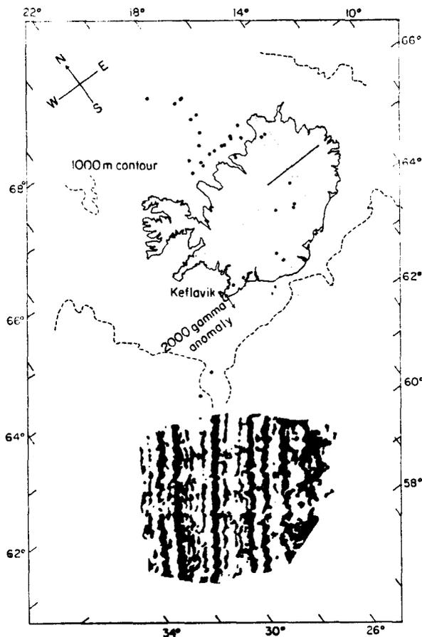
Fig. 1. The magnetic survey area southwest of Iceland. Positive anomalies are shown in solid black. The belts of Quarternary volcanics in Iceland are shaded (after *BODVARSSON and WALKER, 1964*). Epicenters north of the survey area are represented by solid dots (after *SYKES, 1965*). The line in eastern Iceland locates the geologic section used in Fig. 11.
