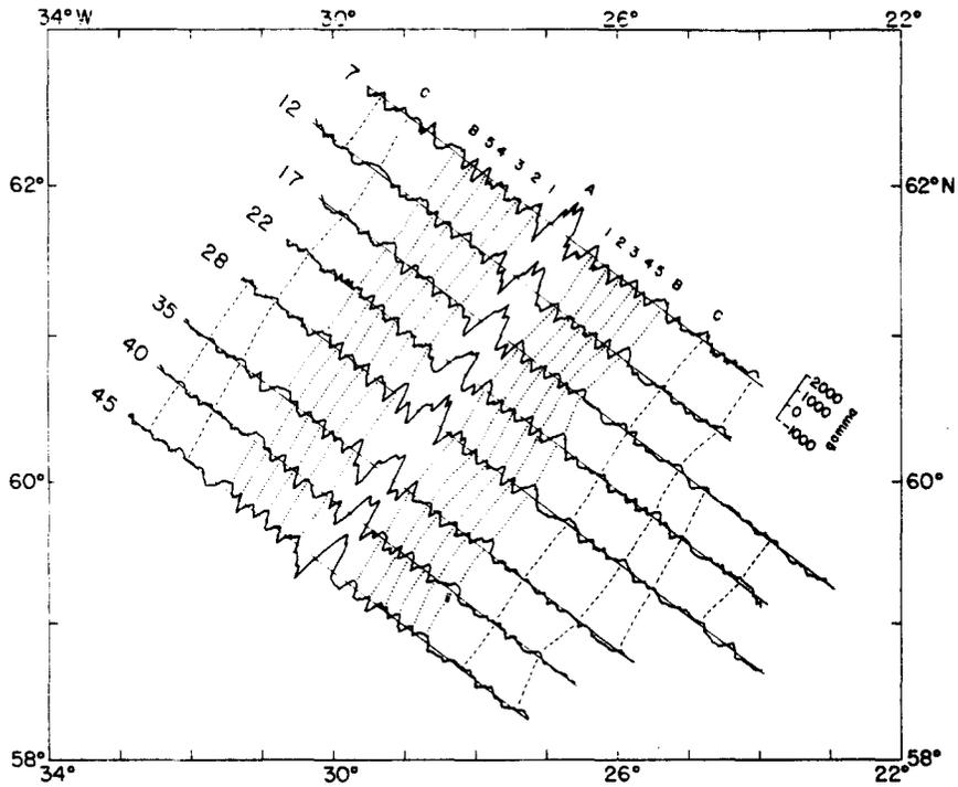
Fig. 3. Eight anomaly profiles projected on lines perpendicular to the structural trends. Profile numbers are at the west end of the lines. Letters and numbers over the anomalies identify particular magnetic features.
