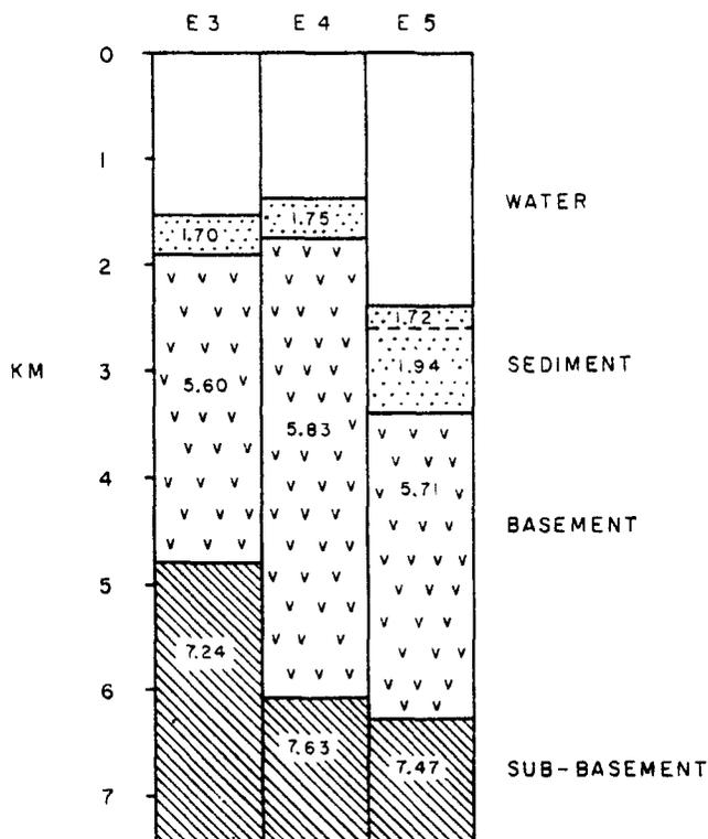
Fig. 8. Seismic refraction sections from EWING and EWING (1959). Velocities are in km/sec.
