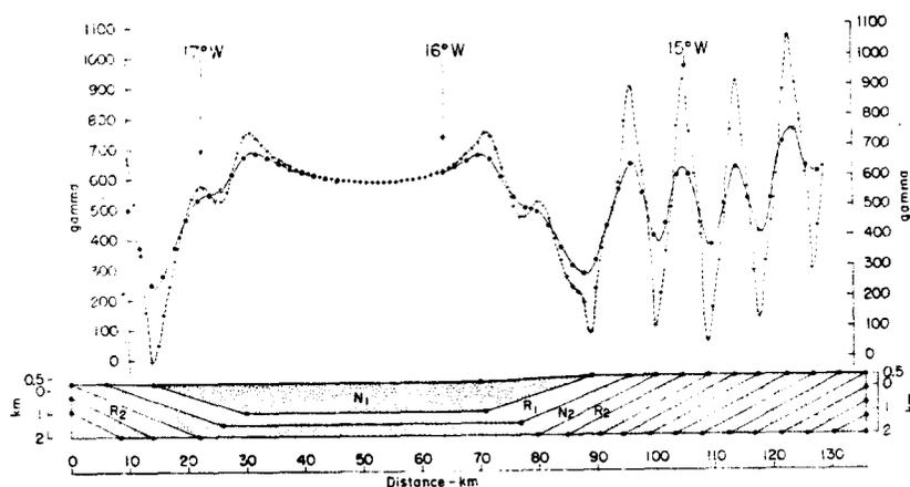
Fig. 11. Calculated anomalies for geologic section of eastern Iceland. "N" and "R" refer to normal and reversely magnetized material. Anomalies are calculated for heights of 1 km (dashed line) and 2.5 km (solid line) above sealevel, or 0.5 km and 2 km above the eastern plateau. The value of magnetization assumed is +0.006 c.g.s. for the normally magnetized material and -0.006 c.g.s. for the reversely magnetized material.
