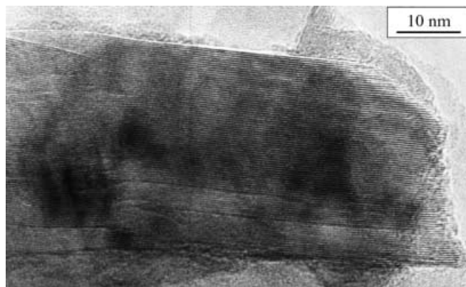
Fig. 9. 002LF image of perfectly stacked aromatic layers in a graphite flake from sample 12. It is impossible to distinguish if such a graphitic lamella derives from the evolution of the microporous phase or from the onion-ring like phase
