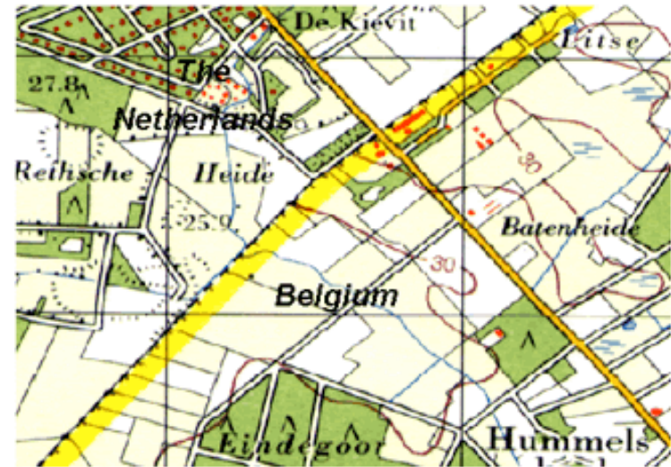
Fragment of the Dutch topo map showing the border of Belgium and the Netherlands. The Mean Sea Level of Belgium differ -2.34m from the MSL of The Netherlands. As a result , contour lines are abruptly ending at the border ( http://www.kartografie.nl ).
