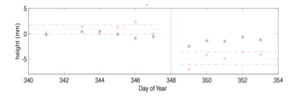
Effect of a radome installation on height (http://facility.unavco.org/ science\_tech/dev\_test/testing/domereport.pdf)
