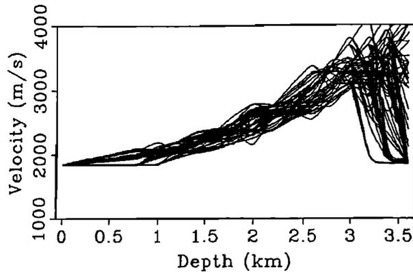
Fig. 5. Plot of 100 velocity models for which the objective function is within 95 % of the maximum. This figure gives an idea of the resolution of the inverse problem.
