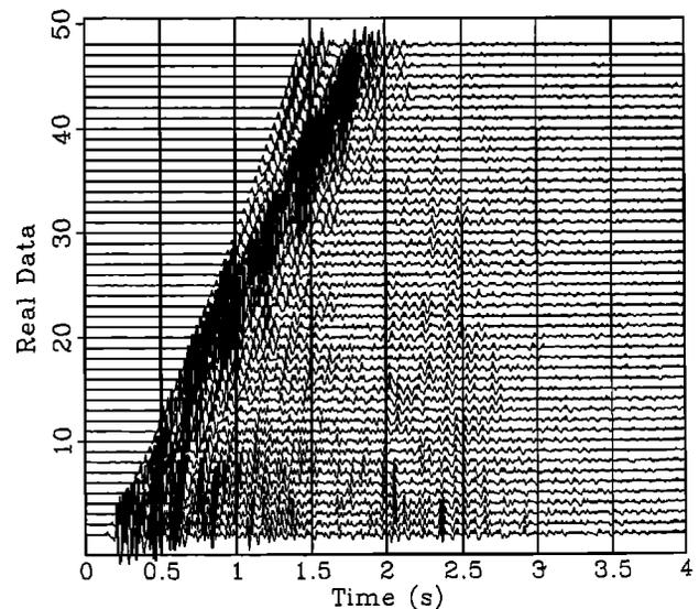
Fig. 1. An example of the 24 shot gathers used for nonlinear velocity inversion. Linear dynamic correction is applied for display.
