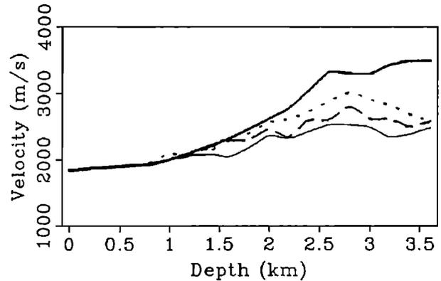
Fig. 4. Velocity models corresponding to the common image gathers in Figure 3. Fine solid line corresponding to Figure 3a, dashed line to Figure 3b, dotted line to Figure 3c and thick solid line to Figure 3d.
