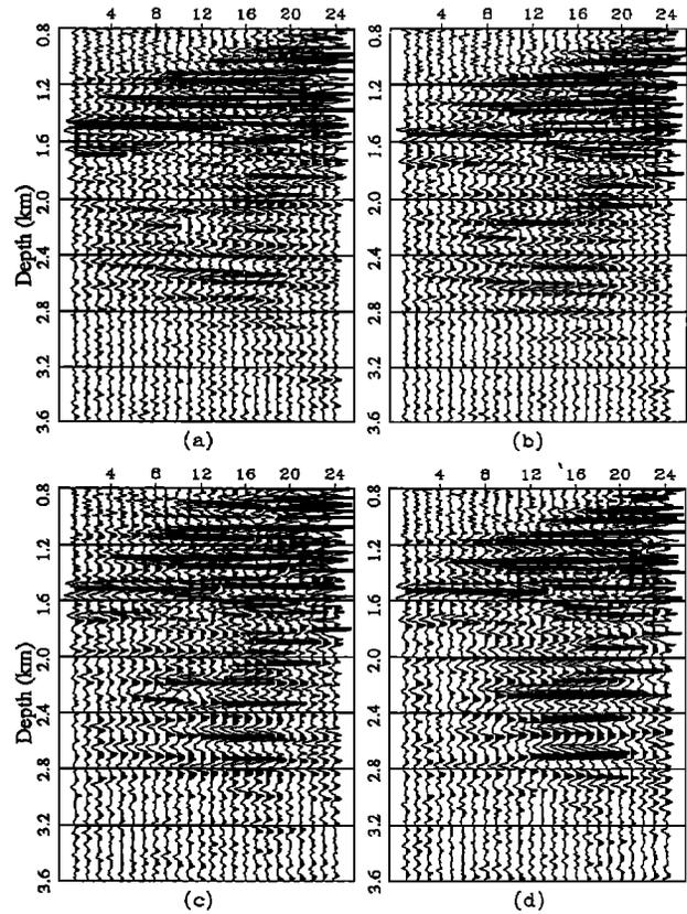
Fig. 3. Image gathers obtained using velocity models that give very different values of the objective function.  $J = 0.3$  for (a),  $J = 0.6$  for (b),  $J = 0.9$  for (c) and  $J = 1.0$  for (d).
