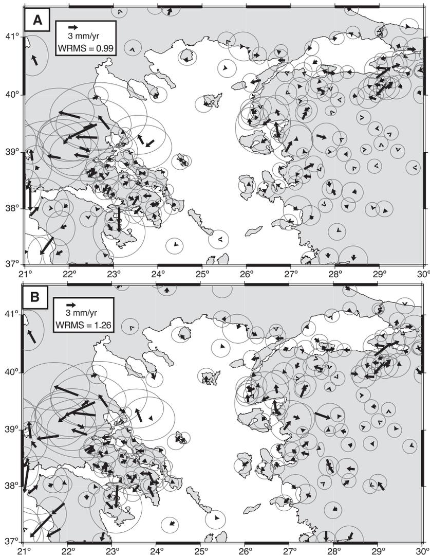
Fig. 5. (A) Residuals between GPS velocities and the fitted model velocities for the GPS-alone model (Fig. 3A). Error ellipses represent 95% confidence intervals. WRMS is weighted root-mean-square. (B) Same as in (A) but for our preferred solution (Fig. 3B).
