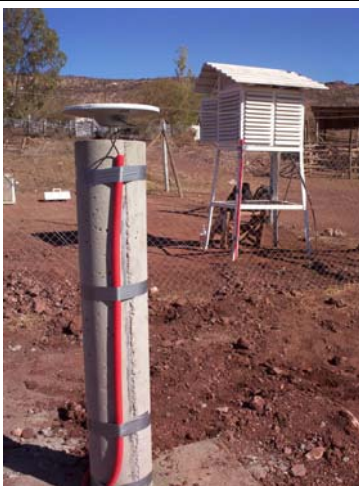
Pillar and receiver shelter
