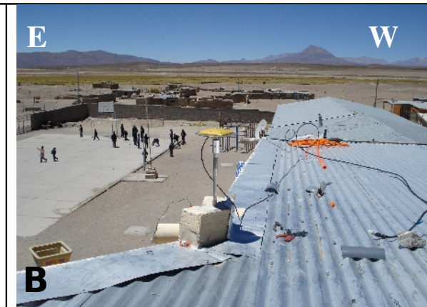
Photography N°6 : Details of the receiver and battery placement. Metallic case (receptor GB-1000 + laptop + 4GB USB pen drive) and plastic case (Battery 80 amp + solar panel regulator)
