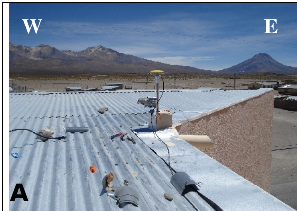
Photography N°5 : Antenna details (tige Delmont and adapter IPGP), cable green (mass antenna connector – land) for electrical storms.
