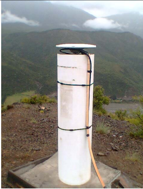
Antenna Trimble Zephyr Geodetic on concrete pilar.
