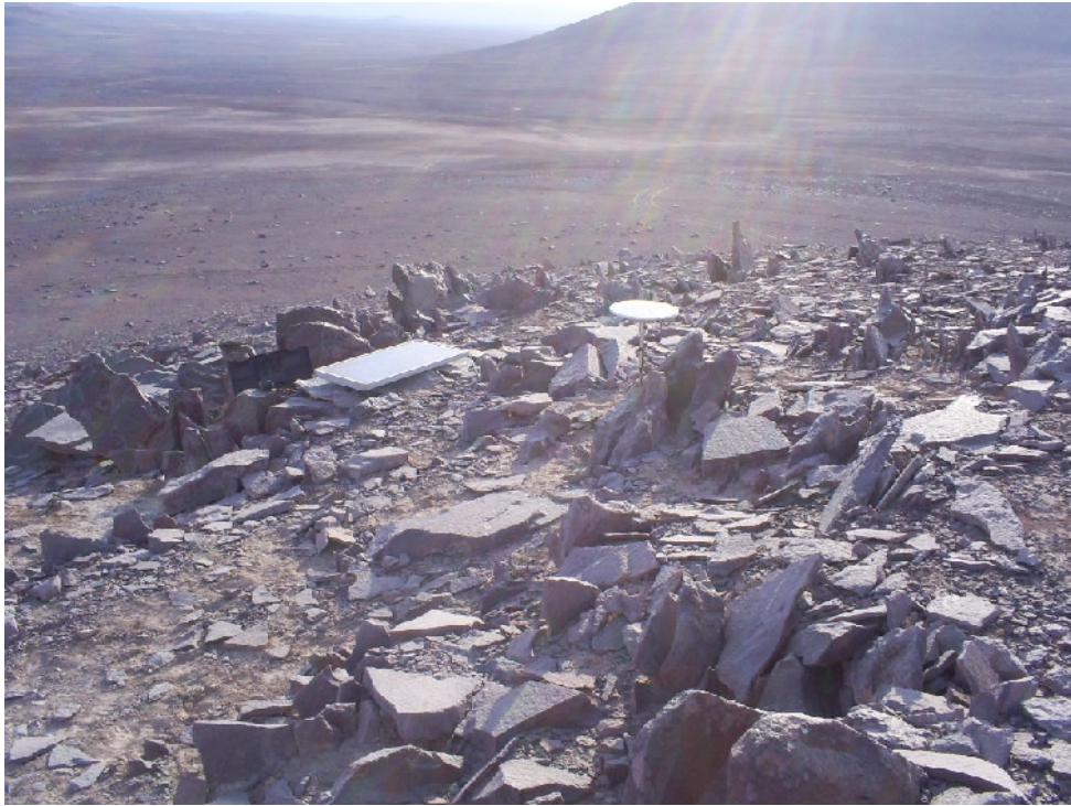
Photography N°2 : MICA receiver placement. The outcrop is characterized by differential erosion produced sub-vertical cornices follow the original stratification planes. No relevant saline-clastic coverture was observed (<5-10 cm).
