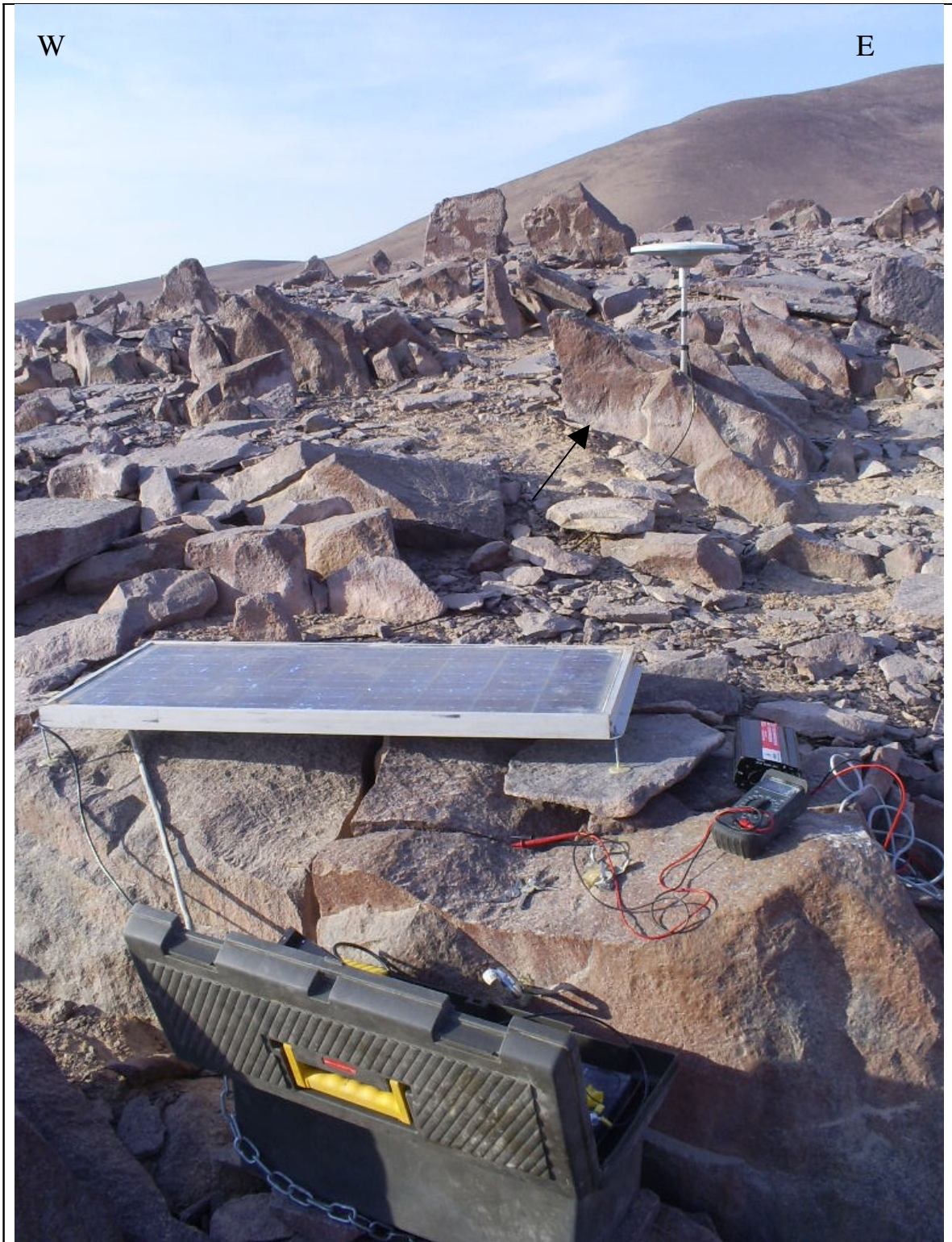
Photography N°1: View of MICA semipermanent station. The cases and solar panel are fixed to the bedrock. Outcrop of Jurassic lava with So? oriented N65W/81NE.
