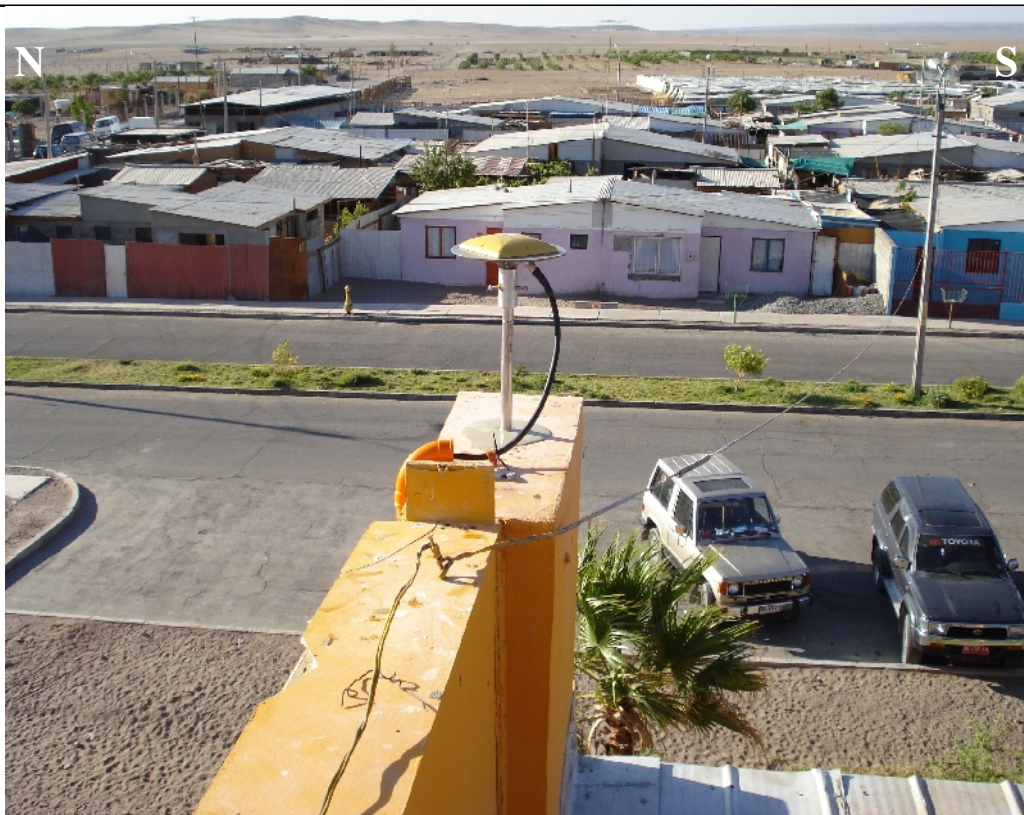
Photography N°2 : Antenna placement detail. (tige Delmont + antenna adapter). Roof made of Zinc material.
