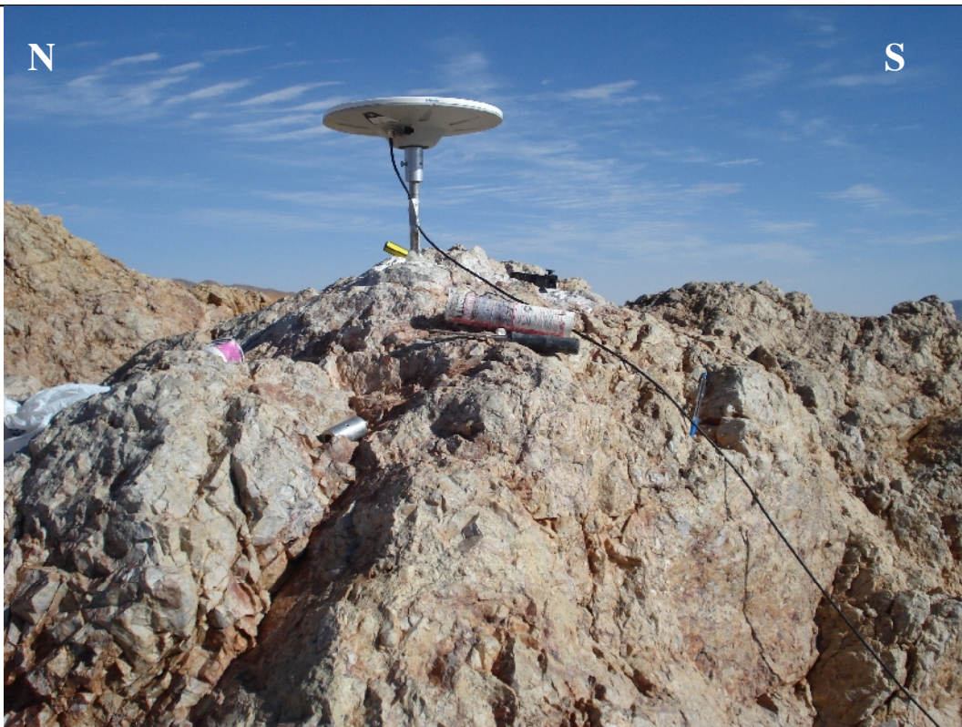
Photography N°2 : Detail of the antenna placement in high silica alteration rocks (tige Delmont + adapter).
