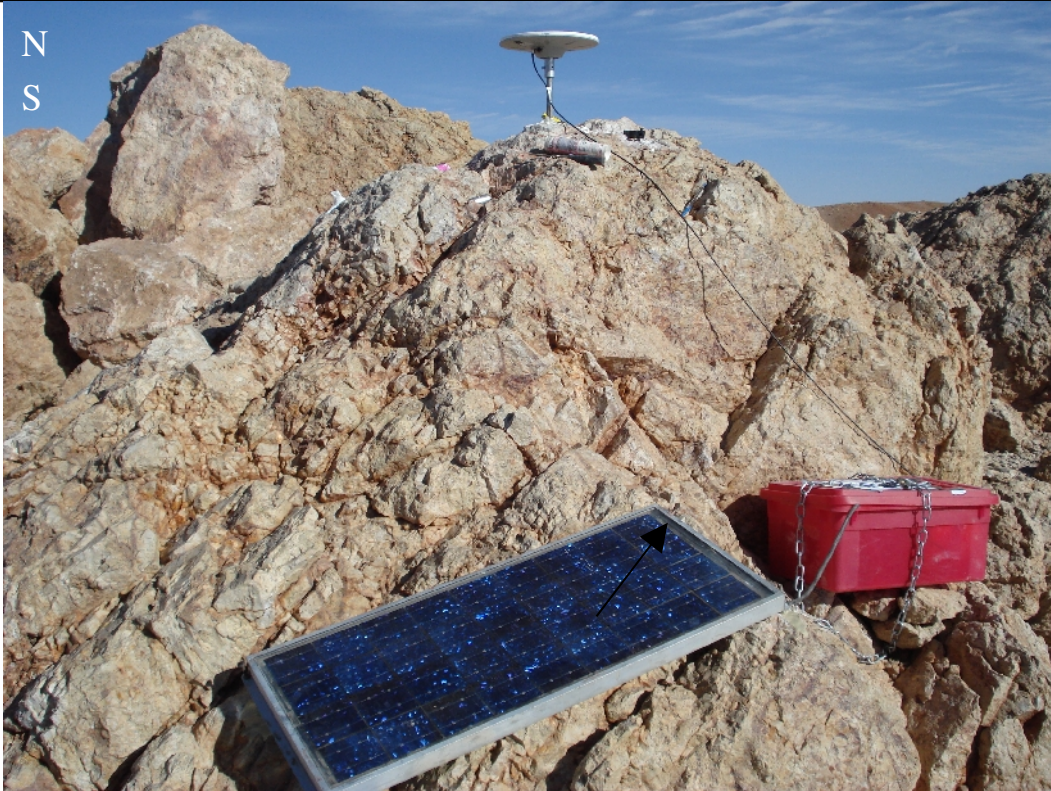
Photography N°1 : View of RADO semipermanent station. The case and solar panel are fixed to the bedrock.
