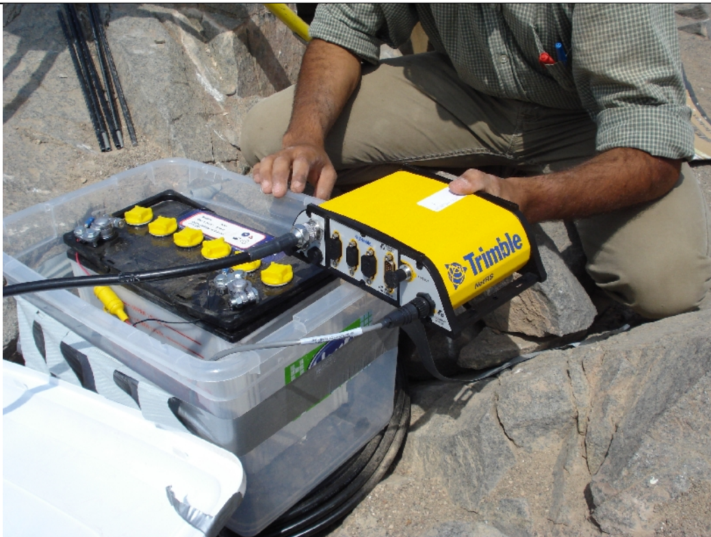
Photography N°4 : Details of the station. Receiver NetRS and battery liquid – 80 AMP
