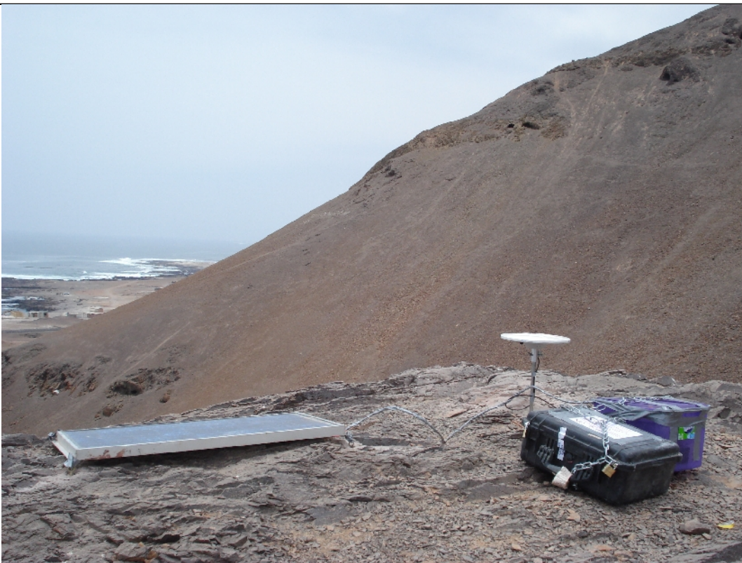
Photography N°2 : The Coastal Cliff (1200 m a.s.l) is located to the east of station producing a relevant shield in the satellite constellation window.
