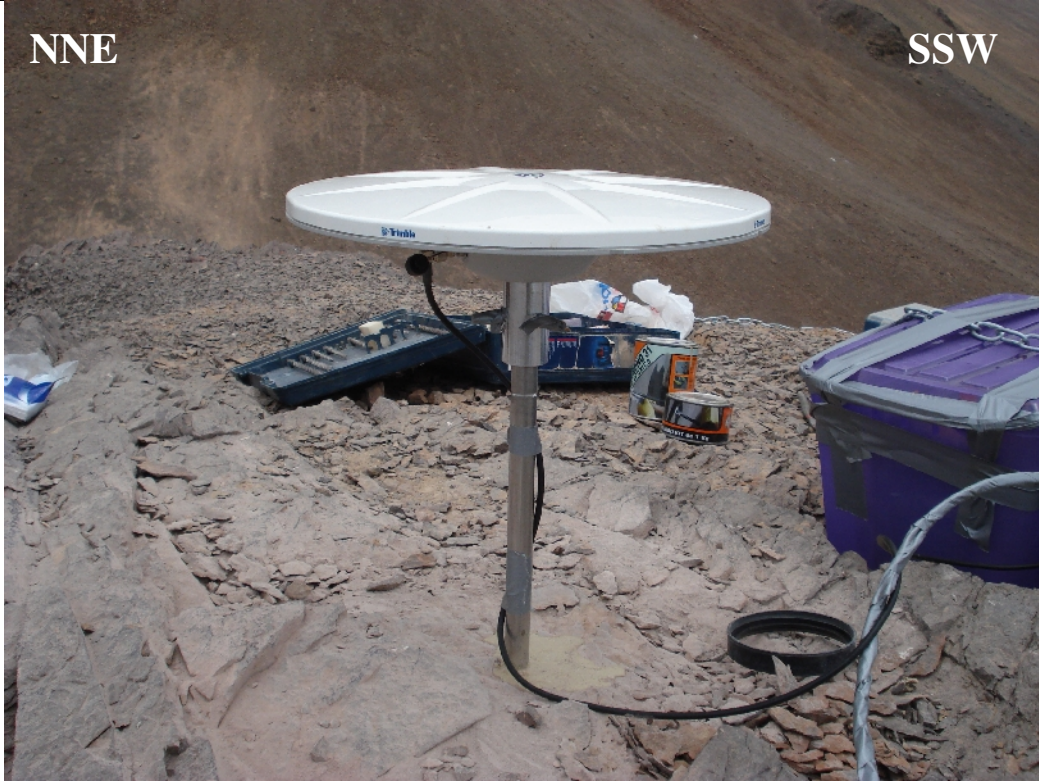
Photography N°3 : Detail of the antenna placement in Jurassic lavas (tige Delmont + adapter).
