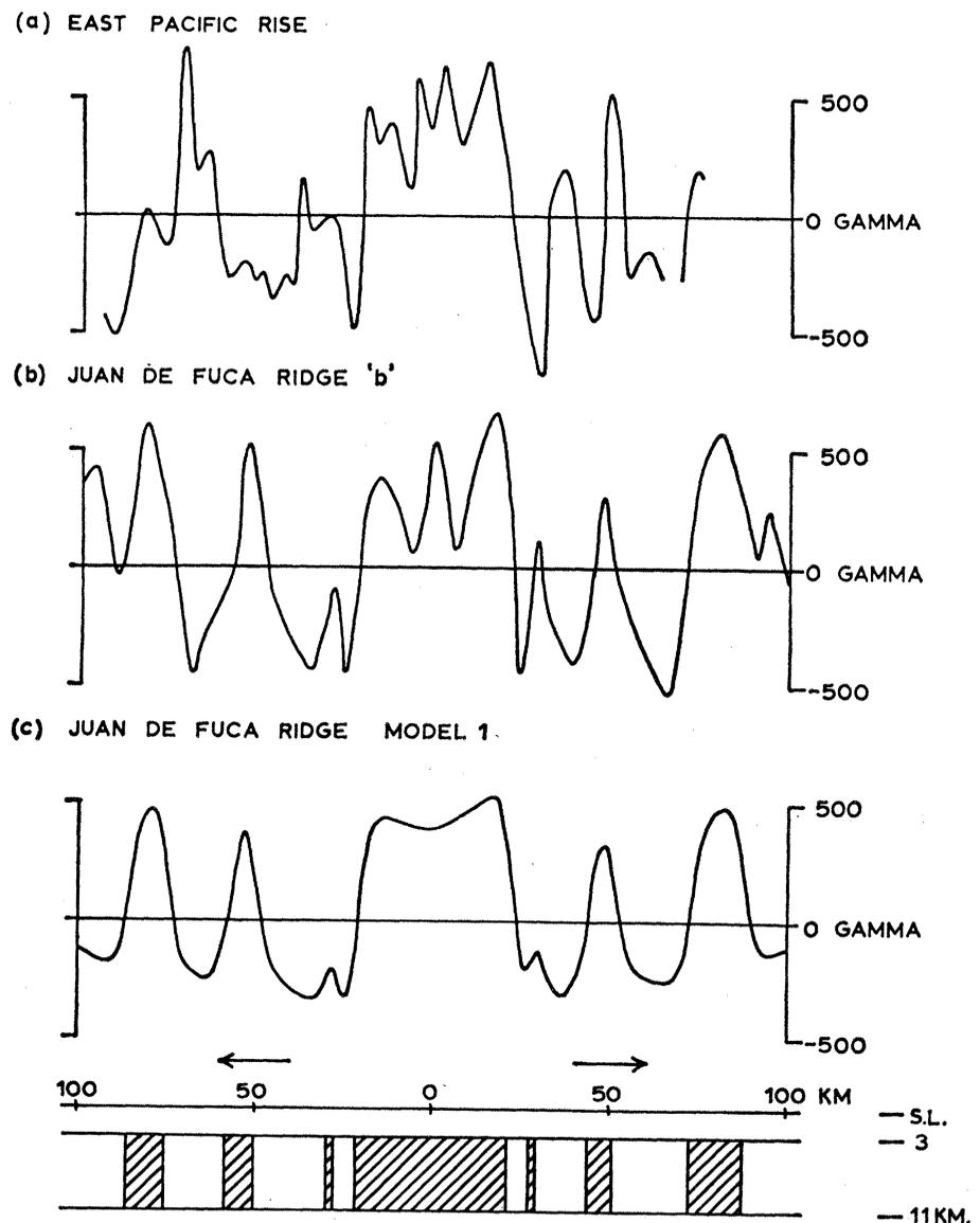
Fig. 2. (a) Observed profile across the East Pacific Rise at 59°S, 149°W (16). (b) Observed profile "b" across the Juan de Fuca Ridge (see Fig. 4). (c) Model and calculated anomaly for Juan de Fuca Ridge, assuming generalized crustal blocks (compare Fig. 1c).
