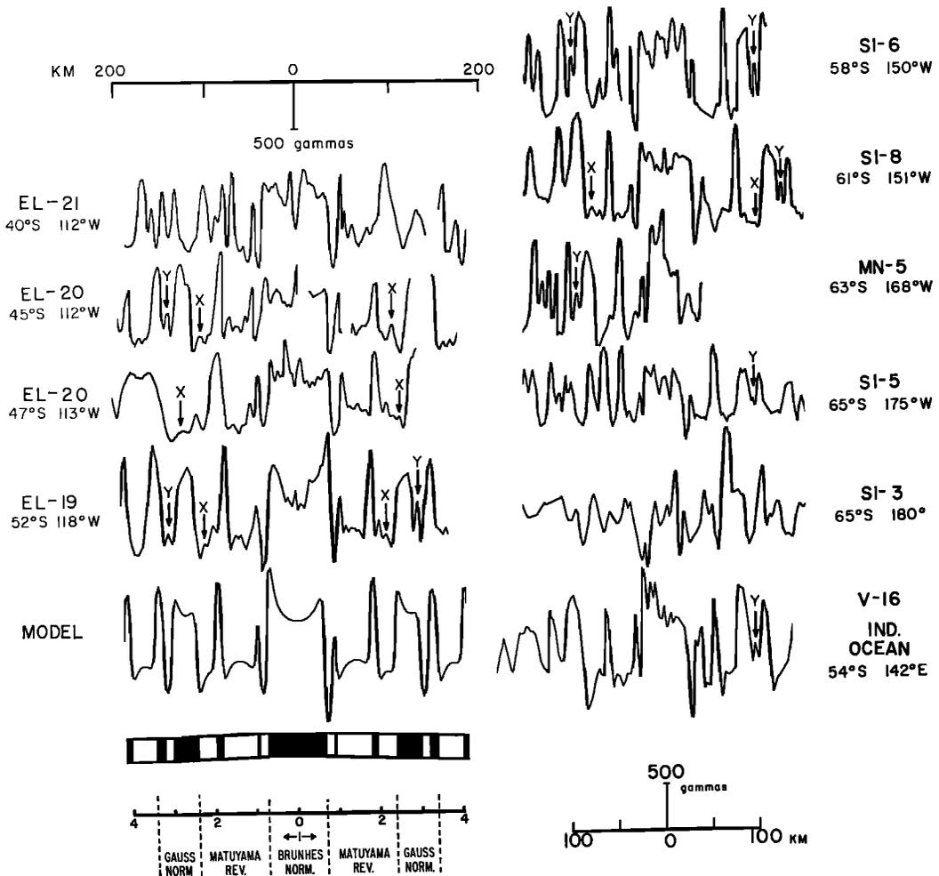
Fig. 7. Ten observed axial magnetic profiles with theoretical profile for known reversals during the last 4 m.y. Anomalies X and Y are not accounted for with the model.
