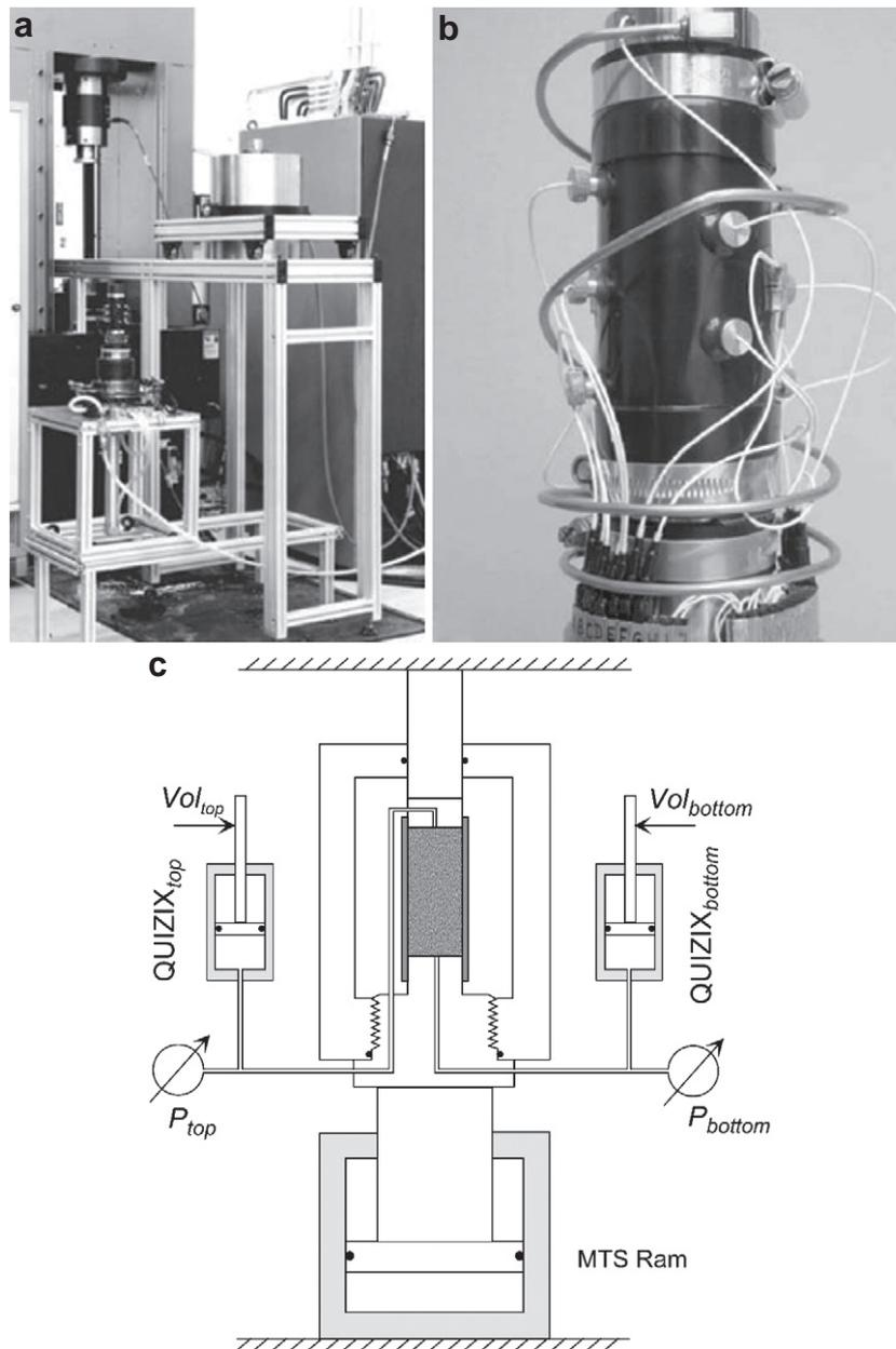
**Fig. 1.** Experimental setup. a) MTS loading frame with 200 MPa pressure vessel. b) Cylindrical specimen encapsulated in rubber jacket with P sensors glued directly on the sample surface. c) Schematic diagram of permeameter/volumometer used for permeability measurements.
