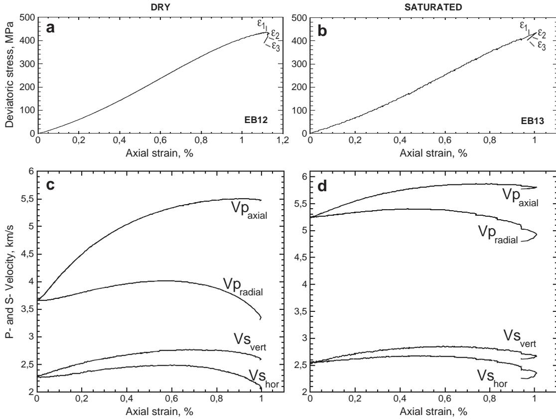
**Fig. 8.** Mechanical data and velocity measurements for the triaxial compression experiment on EB12 done in dry condition and on EB13 done in saturated condition. (a) and (b) deviatoric stress versus axial strain. (c) and (d) P and S wave velocities versus axial strain.
