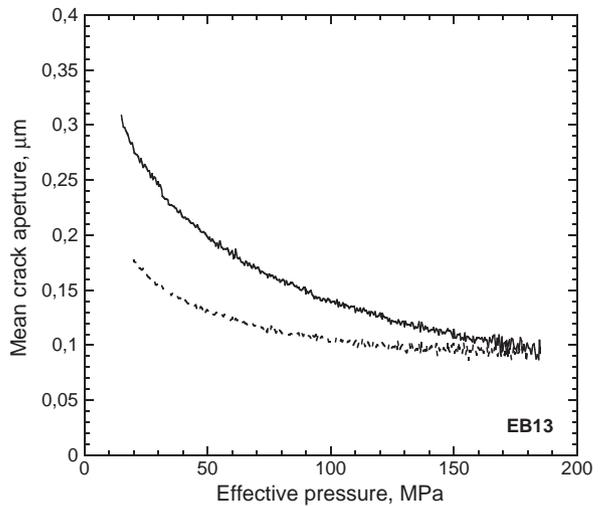
Fig. 6. Evolution of mean crack aperture  $w$  as a function of the effective pressure in the saturated specimen. The mean crack aperture  $w$  is deduced from a combination of i) the permeability data and ii) the crack density  $\rho_i$  and mean crack aspect ratio  $\zeta_i$  obtained by the effective medium model (Fig. 3b and c). The mean crack aperture decreases slightly from 0.3  $\mu\text{m}$  to 0.1  $\mu\text{m}$ . Unloading is shown as dashed line.
