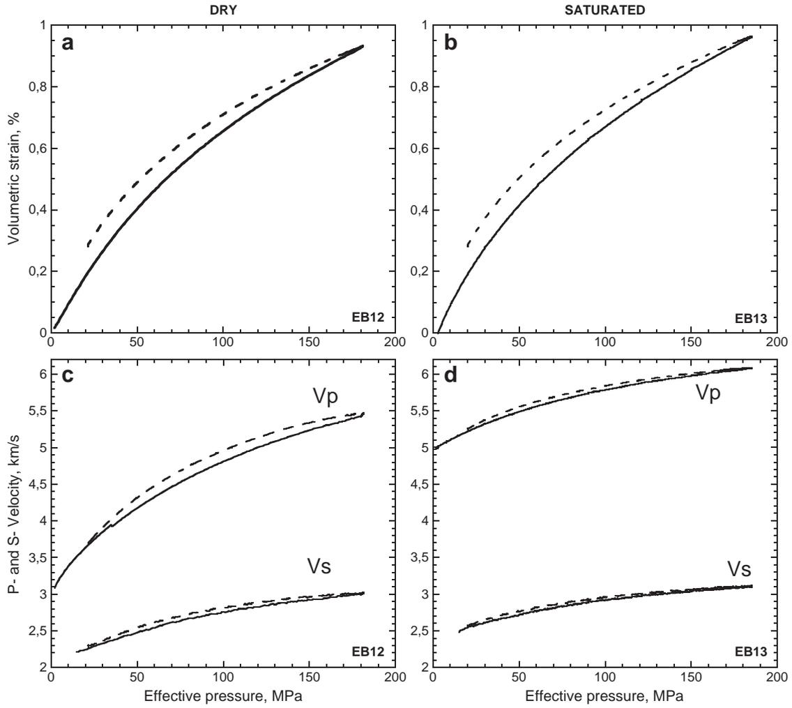
**Fig. 2.** Mechanical data and velocity measurements for the hydrostatic loading on sample EB12 done in dry condition and on sample EB13 done in saturated condition. (a) and (b) Volumetric strain versus effective confining pressure. (c) and (d) *P* and *S* wave velocities versus effective confining pressure. Unloading is plotted as dashed lines.
