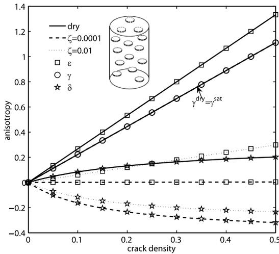
**Figure 3.** Thomsen's anisotropy parameters ( $\gamma$ ,  $\delta$ ,  $\epsilon$ ) as a function of crack density in a dry and a water saturated anisotropic medium. Square symbols correspond to  $\epsilon$ , circles to  $\gamma$  and stars to  $\delta$ . The bold solid line corresponds to the dry case, while the dashed line and grey dotted line correspond to the saturated case with crack aspect ratio of  $10^{-4}$  and  $10^{-2}$  respectively.
