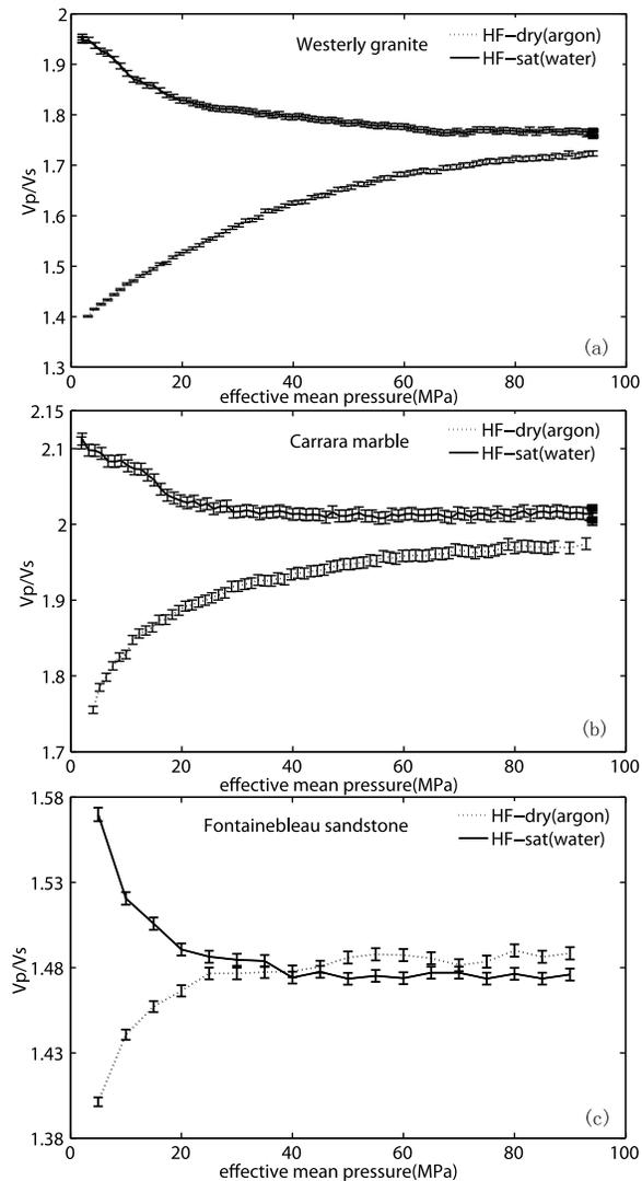
**Figure 1.** Ultrasonic measurements of  $V_p/V_s$  ratio evolution as a function of effective mean pressure of (a) thermally cracked Westerly granite; (b) thermally cracked Carrara marble; (c) 4% porosity Fontainebleau sandstone. The dotted lines indicate measurements performed under argon saturation. The solid lines indicate water saturation case. Error bar has been also shown. Note that these three plots have different vertical scales.
