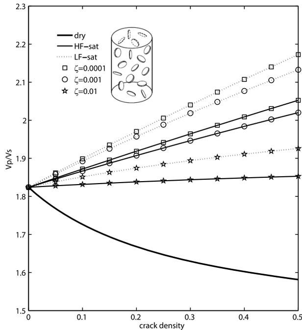
**Figure 2.** Vp/Vs ratio at LF (dotted line) and HF (solid line) plotted versus crack density (range from 0 to 0.5) for a randomly cracked isotropic medium. Curves are given for fixed aspect ratio  $\zeta$  of  $10^{-4}$  (squares),  $10^{-3}$  (circles) and  $10^{-2}$  (stars). The dry case is plotted as a reference (bold solid curve).
